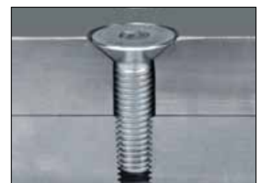
4. Axial relief produced by CBN grinding
