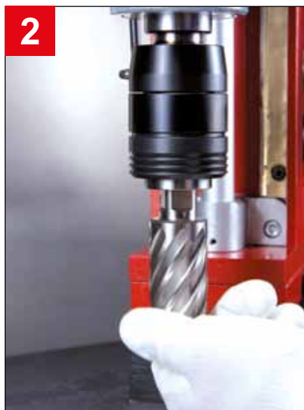
Picture 2: Insert the core drill in the EasyLock. This locks in with a loud "click." The ring spanner snaps down.
