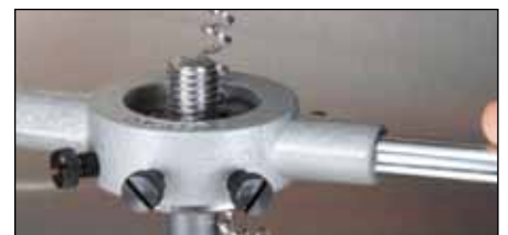
Form B dies = Closed, pre-slotted version!
