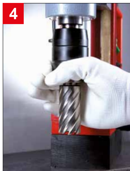
Picture 3: The core drill is fixed securely in the EasyLock. The machine is now ready for operation.
